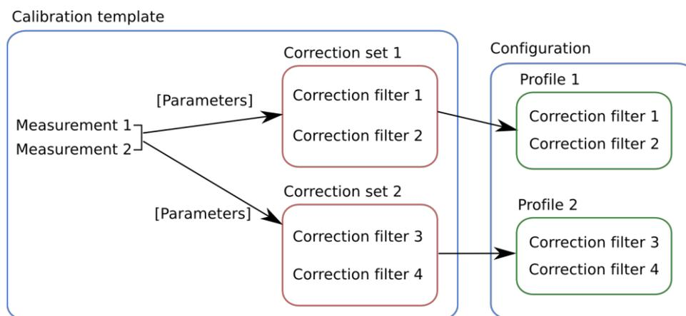
This chapter explains how to create a calibration template and generate correction sets for the *single-amp* speaker configuration modes. To keep the presentation simple, the examples show a single measurement being used for both speakers. Once you are more familiar with DEQX-Cal, you can use a separate measurement for each speaker. (For bi-amp and tri-amp speaker configuration modes, see Chapter 13.)
