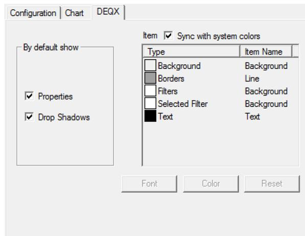
If the **Properties** option is checked, the configuration window displays the parametric room EQ filter settings and the key correction and limit filter parameters (in text). If unchecked, this information is not displayed. It is checked by default.
