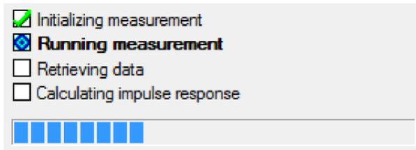
1. "Initializing measurement" uploads the measurement signal to the DEQX.
