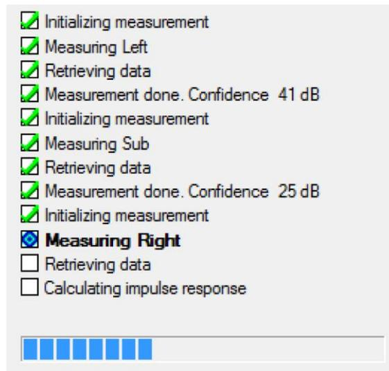
The measurement proceeds in a similar manner as for a speaker measurement, but for each selected speaker and subwoofer in turn.
