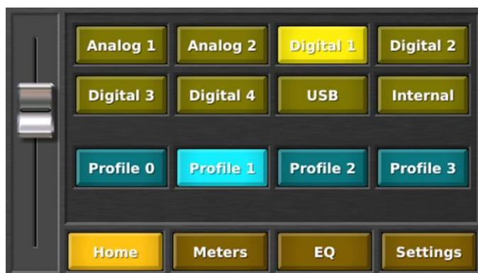
The “Internal” button puts the DEQX (HDP-5 or PreMATE+) into networked streaming audio mode, whereby a networked audio source can be streamed to the DEQX for playback. See Appendix C for full information on this feature. (This is the same as the “Auto” button on the DEQX Remote.)
