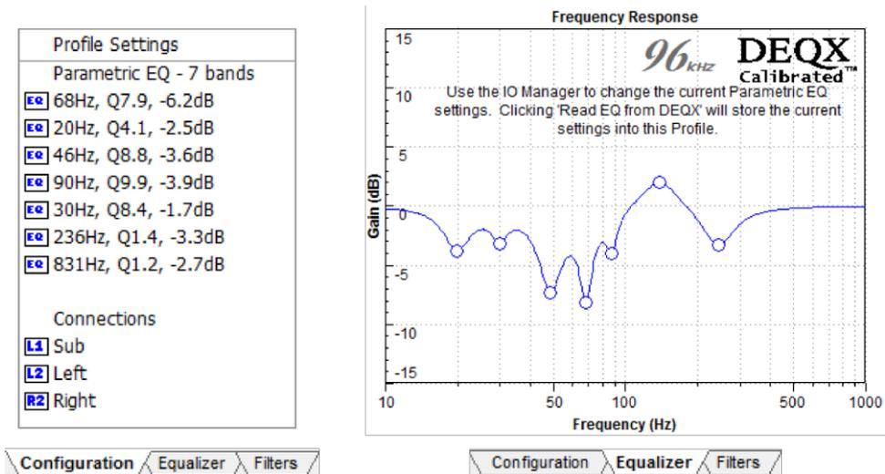
5. If you have changed subwoofer channel levels in the IO Manager, adjust gain in the Filter Properties dialog box of each subwoofer by the same amount. After doing this, return to the IO Manager and reset the channel gains back to zero.
