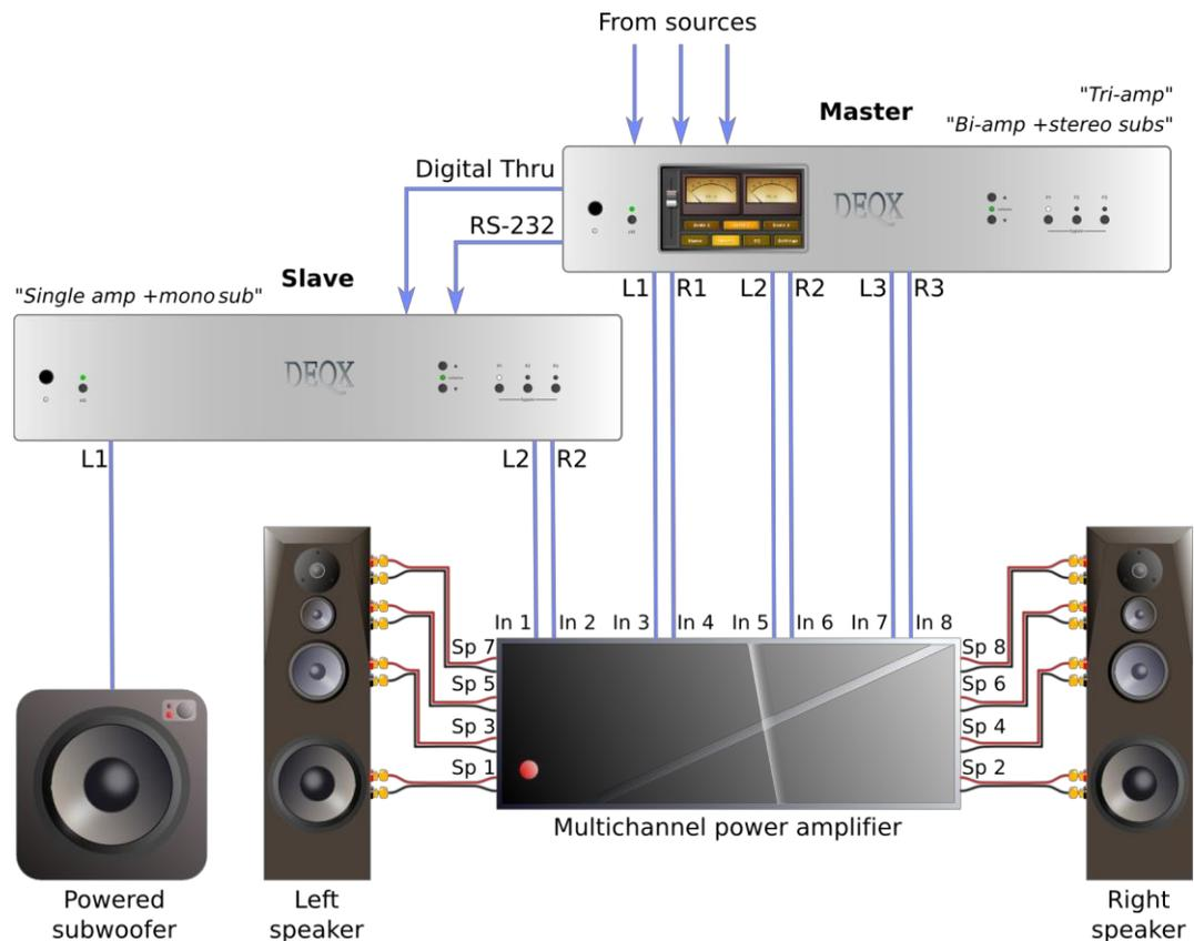
Figure 9. Multi-way active speaker with master and slave DEQX
