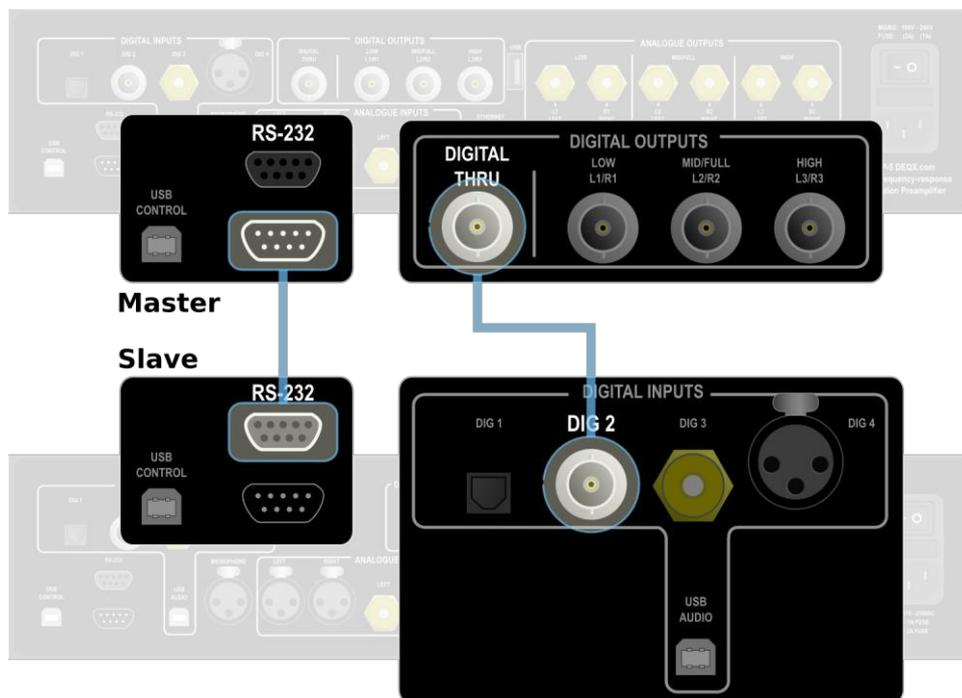
Figure 8. Connections between master and slave DEQX units
