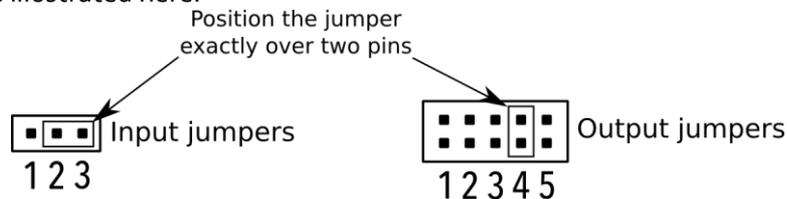
Do **not** force jumpers – they will slide easily when positioned correctly.
