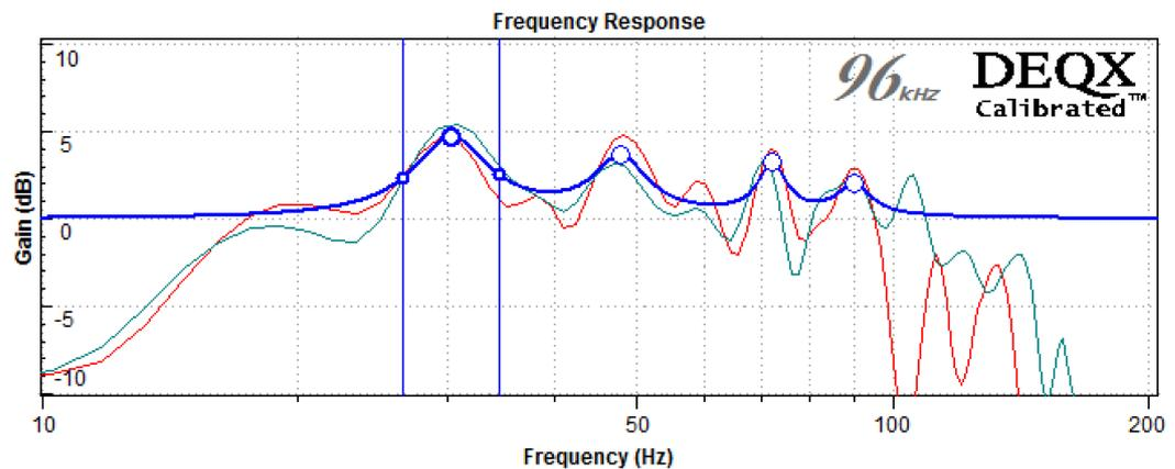
Then click the **Invert EQ** button to obtain the “right way up” EQ curve as shown on the previous page. (If you use this method, be sure to always set the EQ curve to the correct orientation before re-measuring or listening to the effect of the EQ.)
