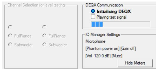
When the indicator changes to “Playing test signal,” adjust the measurement signal level as described on page 50. For a room measurement, however, the input level should typically be peaking in the range of 75–85 dB.
