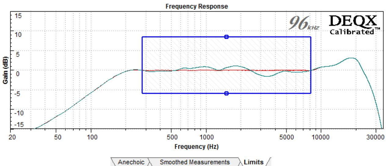
You can also double-click on the limits rectangle to bring up a dialog box that allows you to enter the limits directly (shown at right). As a general rule, increasing Max Boost beyond the default of 6 dB is not recommended.
