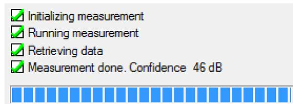
For a speaker measurement, the confidence level should always be greater than 20 dB. If it is not, you will need to retry the measurement (see next page). Increasing the number of sweeps, increasing the sweep length, reducing background noise, and increasing the signal level (but not so far as to introduce distortion) are all ways to improve the confidence level of the measurement.
