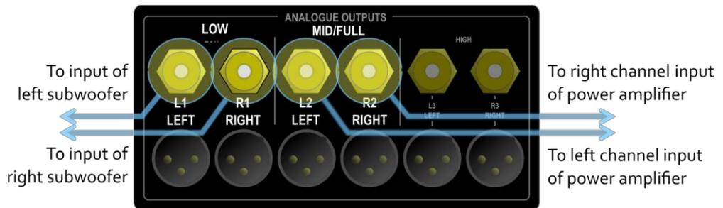
In the case of the PreMATE, PreMATE+, HDP-4 and HDP-5, use the balanced outputs if the connected amplifiers or subwoofers have balanced inputs.
