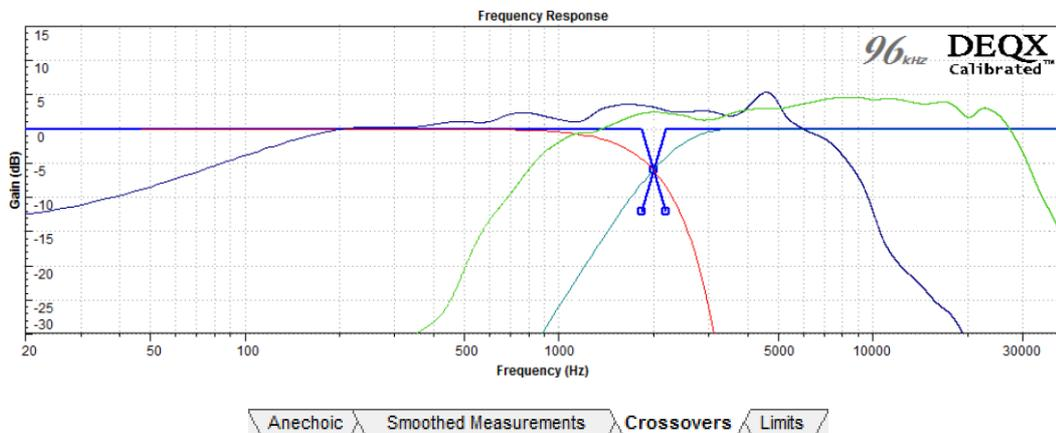
To change the crossover frequency, drag the central control point (below left). To change the crossover slope, drag one of the two lower control points to the left or right. Alternatively, double-click on the crossover control to bring up a dialog that allows you to enter the frequency and slope directly (below right).
