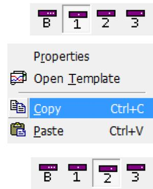
After copying settings, visually check the configuration to confirm that the data has been copied.
