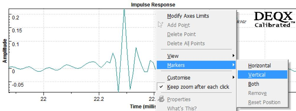
Right-click on the plot and select "Markers" then "Vertical." Place one of the markers at the impulse response peak. In this example, the delay of the speaker is 22.3 ms:
