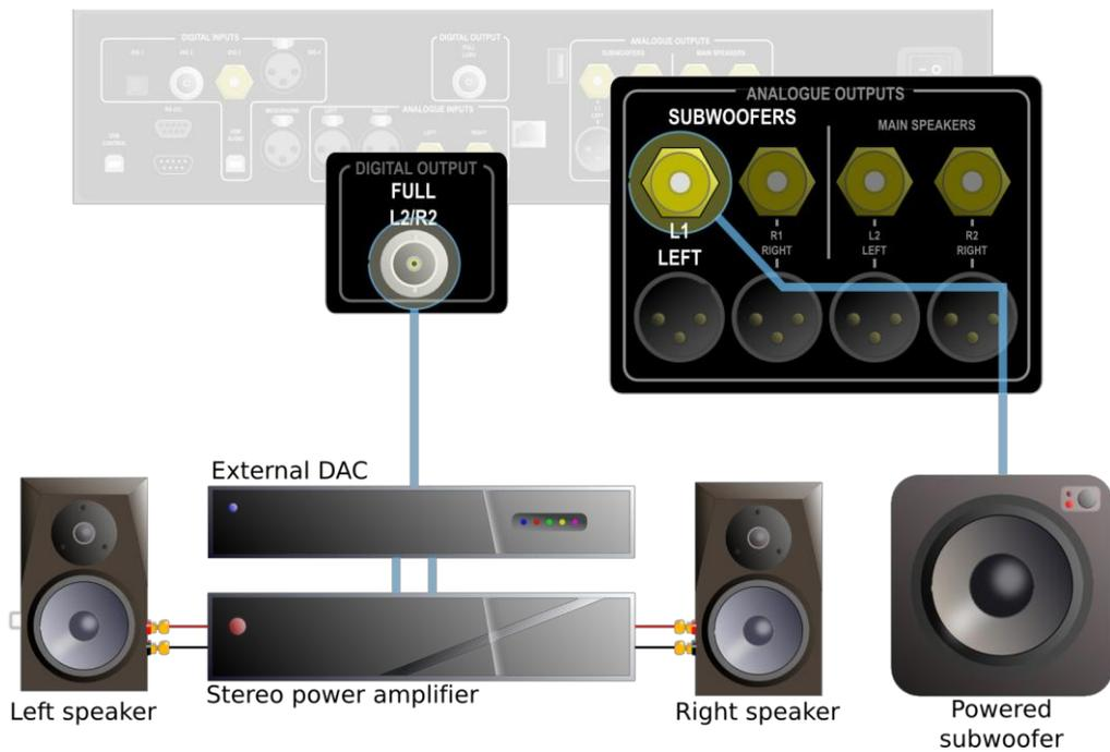
The diagram above illustrates the use of the digital output of the PreMATE or PreMATE+. Connect the digital output, labeled **Full L2/R2**, to an external DAC via a BNC cable (or an RCA cable with a BNC-RCA adapter). The outputs of the DAC are connected to the power amplifier, which in turn drives the left and right speakers. Note that the external DAC must be capable of decoding a 24-bit 96 kHz signal.
