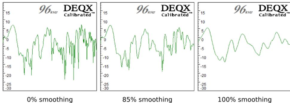
In addition to the individual adjustment for each plot, all selected plots can have their smoothing changed with the slider at the left of the viewer toolbar.
