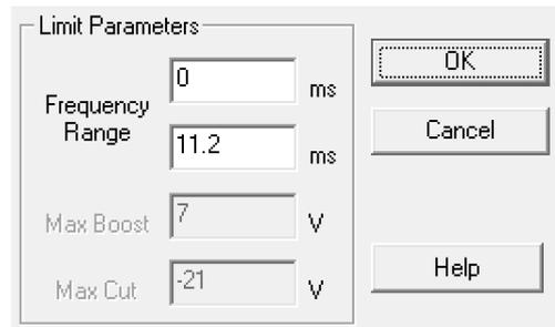
The *effective length* of the time window is the time difference between the impulse response peak and the vertical bar. In the example below, the impulse response peak occurs at 5.7 ms and the bar is set at 11.2 ms. Therefore, the effective window length is  $(11.2 - 5.7) = 5.5$  ms. The effective window length determines the frequency resolution and thus the lowest correction frequency, as given by Table 3 on page 58.
