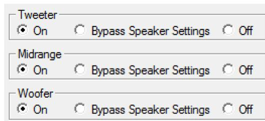
While normally left at "On," setting a driver to "Bypass Speaker Settings" sends the unfiltered signal to that driver. Setting it to "Off" turns off that driver.
