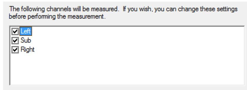
Usually, you will run the room measurement on all enabled outputs. You can select and deselect specific channels with the checkboxes if you wish.
