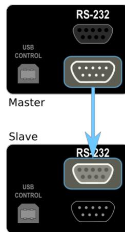
With the PC connected to the slave DEQX unit and DEQX-Cal running, open the Options dialog to disable the slave’s front panel and remote control (see page 151). This ensures that the master is the only unit that responds directly to user input:
