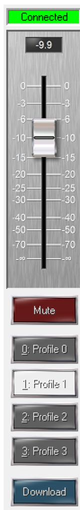
At the left of the Control Panel is a strip that displays the master volume slider and profile selectors. The status indicator at the top is green if DEQX-Cal detects connection to the DEQX. It turns red if clipping is detected (page 135).
