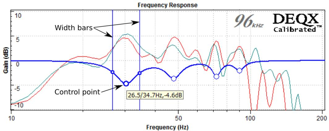
In this example, the EQ curve is set to "pull the peaks down." This can be done because the subwoofers' **Scale** has been set so that their baseline is at about 0 dB.
