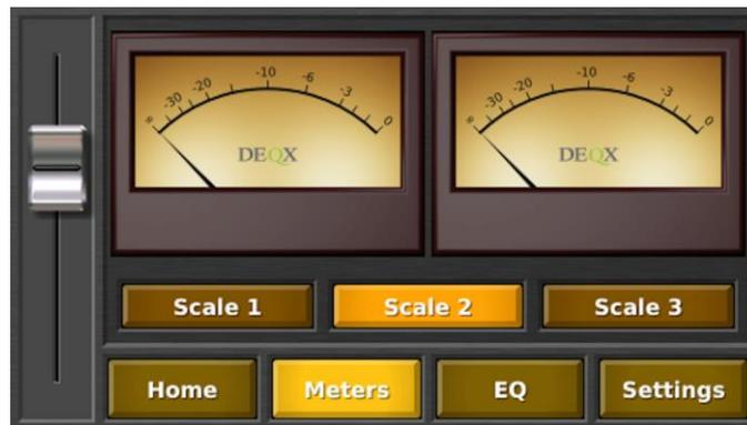
Note that the touchscreen display does not go to sleep when the Meters screen is displayed.
