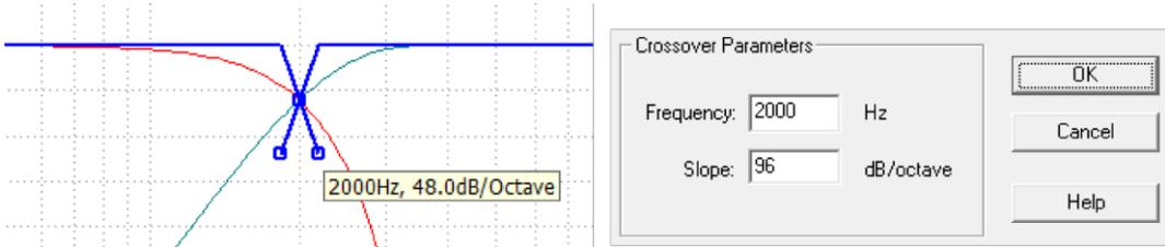
Hovering the mouse over a control point will display the crossover frequency and slope. The frequency and slope are also displayed above the plot area, together with the delay introduced by that choice of frequency and slope, and the maximum allowed delay.
