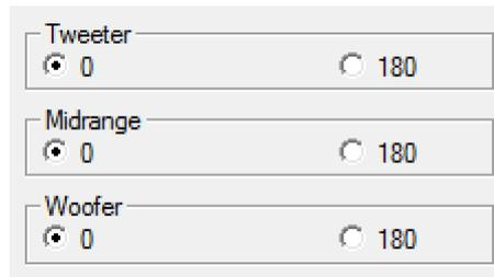
Note: during testing of a speaker, the individual outputs can be inverted in the IO Manager. However, for permanent storage into a configuration, any polarity inversion must be set on this tab.
