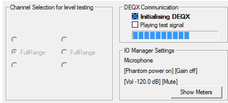
When the screen switches to the “Playing test signal” indicator, switch to the IO Manager to view the meters. (Click the **Show Meters** button if it is not visible.)
