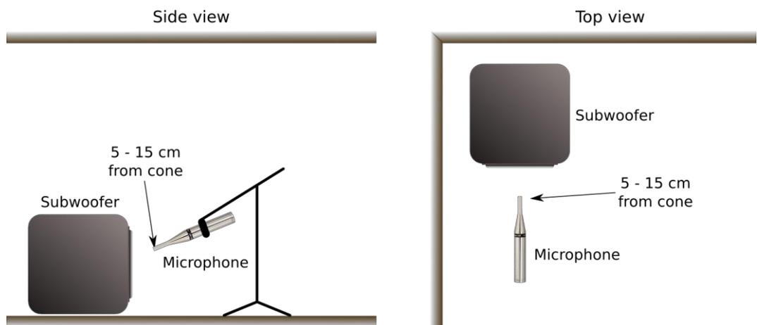
Figure 2. Subwoofer measurement setup
