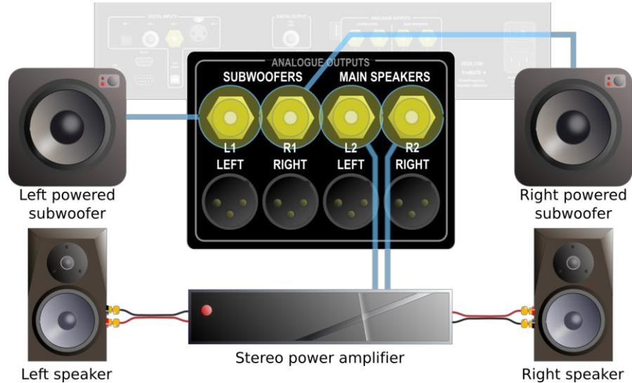
The diagram above illustrates the connections for a pair of full range speakers and a pair of stereo subwoofers connected to a PreMATE or PreMATE+. Take the left channel speaker output from **L2** and the right channel speaker output from **R2**. Connect the left and right subwoofers to **L1** and **R1** and in DEQX-Cal, set the speaker configuration mode to "Single amp with optional stereo subwoofers."
