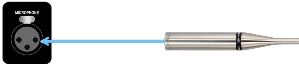
Each microphone supplied with a DEQX Calibration Kit has a unique calibration file, identified by the serial number printed on the microphone. The calibration file must be loaded into DEQX-Cal for accurate results.
