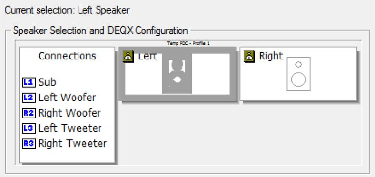
**Screen 6.** Any of the (two or three) drivers can be selected for test signal playback (left-hand side of the example screenshot below). The woofer is the default, but a different driver can be selected by clicking on its radio button. This will result in a short pause while a new test signal is uploaded to the DEQX. The test signal will then resume from the selected driver.
