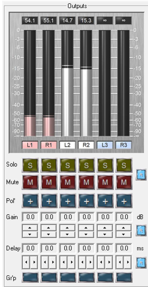
The buttons underneath the meters modify the output signal for each channel. These controls are intended for use in testing, prototyping, and speaker design work.
